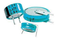
Type EDC electric double layer supercapacitors offer high capacitance values in a thru hole stacked coin type package. Primarily designed for integrated circuit voltage backup, the capacitors can also be used to deliver the initial power from batteries.
