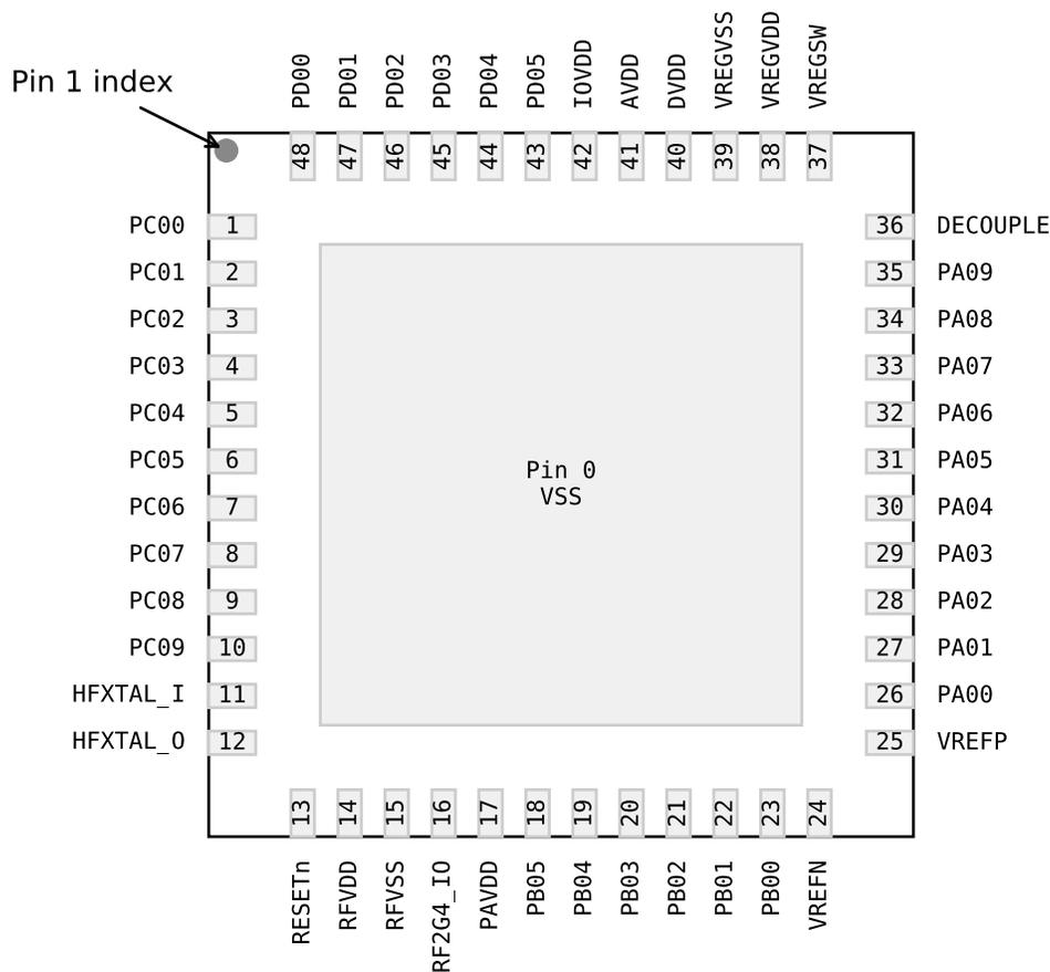
Figure 6.1. QFN48 / Standard Device Pinout
