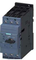
CIRCUIT BREAKER, SIZE S2, FOR MOTOR PROTECTION, CLASS 10, A-RELEASE 22...32A, N-RELEASE 416A, SCREW TERMINAL, INCREASED SWITCHING CAPACITY
