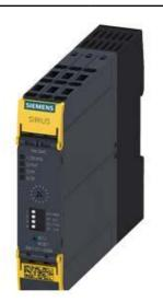
SIRIUS SAFETY RELAY BASIC UNIT ADVANCED SERIES WITH TIME DELAY 0.05-3S RELAY ENABLING CIRCUITS 2 INSTANTANEOUS NO CONTACTS 2 DELAYED NO CONTACTS US = 24 V DC SPRING-LOADED TERMINAL
