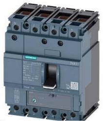
CIRCUIT BREAKER 3VA1 IEC FRAME 160 BREAKING CAPACITY CLASS N ICU=25KA @ 415 V 4-POLE, LINE PROTECTION TM220, ATFM, IN=20A OVERLOAD PROTECTION IR=14A ...20A SHORT CIRCUIT PROTECTION II=10 X IN NEUTRAL UNPROTECTED CABLE CONNECTION
