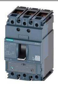
CIRCUIT BREAKER 3VA1 IEC FRAME 160 BREAKING CAPACITY CLASS N ICU=25KA @ 415 V 3-POLE, LINE PROTECTION TM240, ATAM, IN=25A OVERLOAD PROTECTION IR=17,5A ...25A SHORT CIRCUIT PROTECTION II=5...10 X IN BUSBAR CONNECTION
