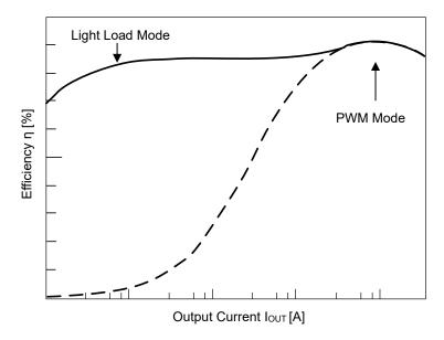
Figure 30. Efficiency (Light Load Mode, PWM Mode)
