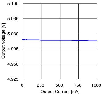
Figure 87. Load Regulation (V<sub>IN</sub> = 12 V)
