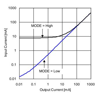
Figure 77. Input Current vs Output Current  $(V_{IN} = 12 V)$
