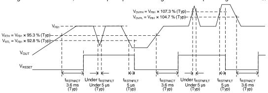
Figure 34. Reset Timing Chart (BD9P105MUF-C)
