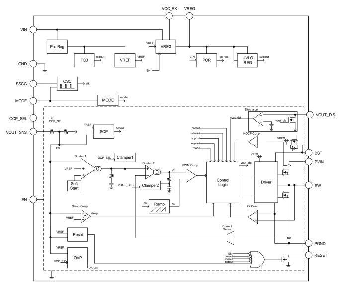
Figure 8. Block Diagram (BD9P135MUF-C, BD9P155MUF-C)
