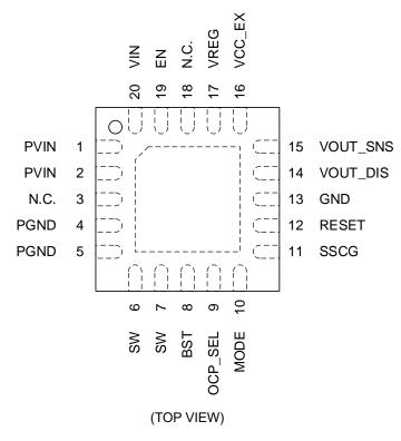
Figure 5. Pin Configuration (BD9P135MUF-C, BD9P155MUF-C)
