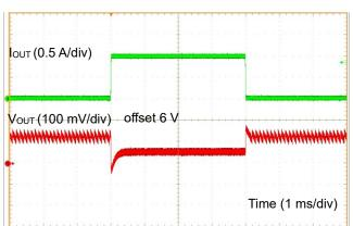
Figure 54. Load Response 1 (V<sub>IN</sub> = 12 V, V<sub>MODE</sub> = 5 V, I<sub>OUT</sub> = 0 A to 1 A)
