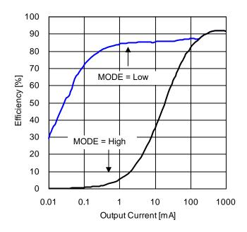
Figure 76. Efficiency vs Output Current (V<sub>IN</sub> = 12 V)
