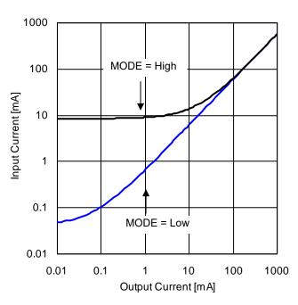
Figure 51. Input Current vs Output Current (V<sub>IN</sub> = 12 V)
