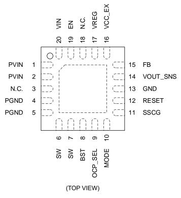
Figure 6. Pin Configuration (BD9P105MUF-C)
