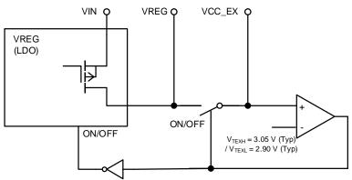
Figure 38. VCC EX Block Diagram
