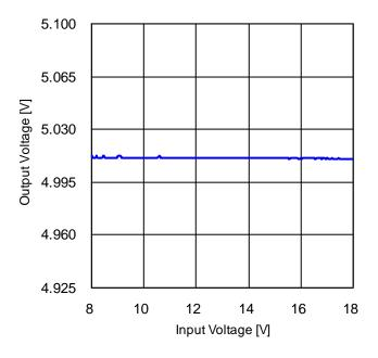
Figure 86. Line Regulation (I<sub>OUT</sub> = 1 A)
