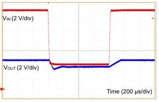
Figure 56. Line Response 1 ( $V_{IN}$  = 16 V to 8 V,  $I_{OUT}$  = 1 A)
