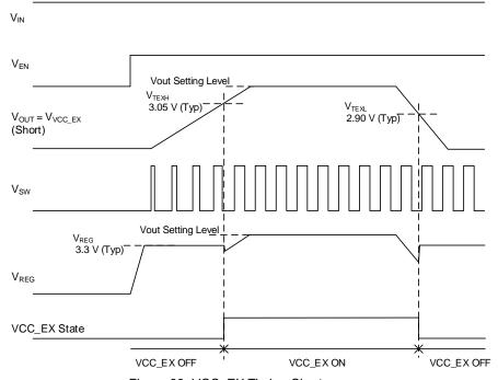
Figure 39. VCC\_EX Timing Chart
