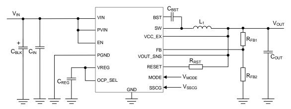
Figure 47. Application Sample Circuit
