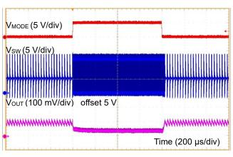
Figure 79. MODE ON/OFF Response (V<sub>IN</sub> = 12 V, I<sub>OUT</sub> = 50 mA)
