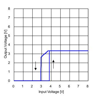
Figure 72. Output Voltage vs Input Voltage 2  $(R_{LOAD} = 3.3 \Omega)$
