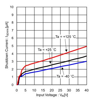
Figure 9. Shutdown Current vs Input Voltage
