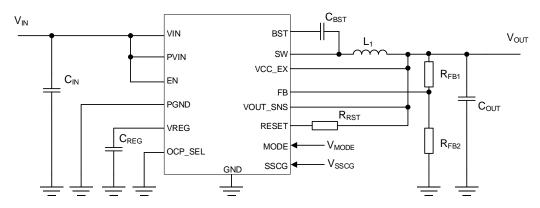
Figure 3. Application Circuit (BD9P105MUF-C)
