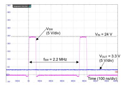
Figure 29. Switching Waveform ( $V_{IN} = 24 \text{ V}$ ,  $V_{OUT} = 3.3 \text{ V}$ ,  $I_{OUT} = 0.5 \text{ A}$ ,  $f_{SW} = 2.2 \text{ MHz}$ )
