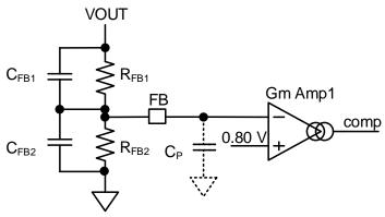
Figure 48. Setting for Output Setting Resistor
