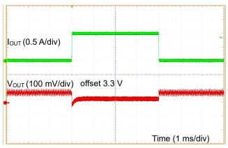
Figure 67. Load Response 1 ( $V_{IN}$  = 12 V,  $V_{MODE}$  = 5 V,  $I_{OUT}$  = 0 A to 1 A)
