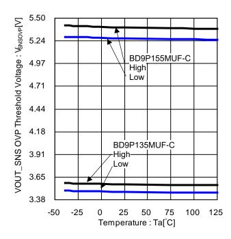
Figure 28. VOUT\_SNS OVP Threshold Voltage vs Temperature (BD9P135MUF-C/BD9P155MUF-C)
