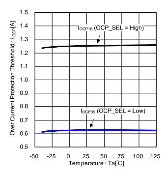
Figure 20. Over Current Protection Threshold vs Temperature
