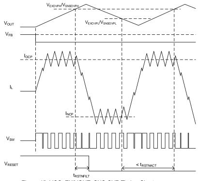
Figure 45. VCC\_EX/VOUT\_SNS OVP Timing Chart
