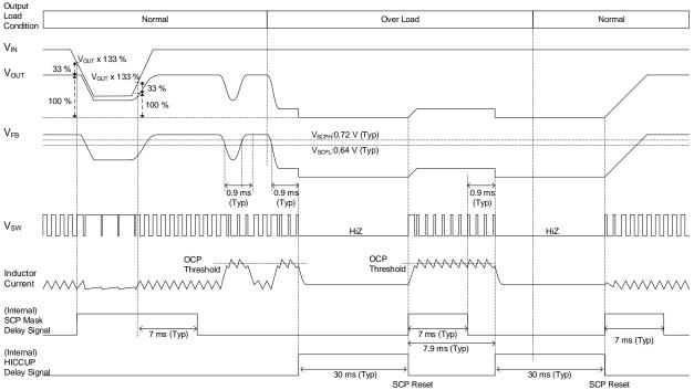
Figure 41. Short Circuit Protection (SCP) Timing Chart (BD9P105MUF-C)
