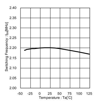
Figure 19. Switching Frequency vs Temperature
