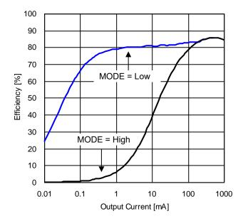
Figure 63. Efficiency vs Output Current  $(V_{IN} = 12 V)$
