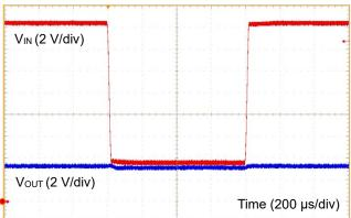
Figure 69. Line Response 1 (V<sub>IN</sub> = 16 V to 8 V, I<sub>OUT</sub> = 1 A)
