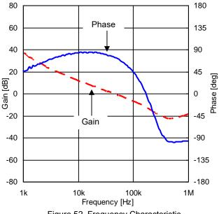
Figure 52. Frequency Characteristic  $(V_{IN} = 12 \text{ V}, I_{OUT} = 0.5 \text{ A})$
