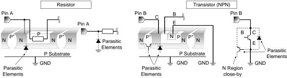
Figure 93. Example of Monolithic IC Structure
