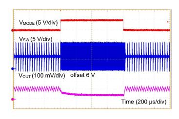
Figure 53. MODE ON/OFF Response  $(V_{IN} = 12 \text{ V, } I_{OUT} = 50 \text{ mA})$
