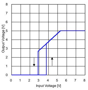
Figure 85. Output Voltage vs Input Voltage 2  $(R_{LOAD} = 5 \Omega)$
