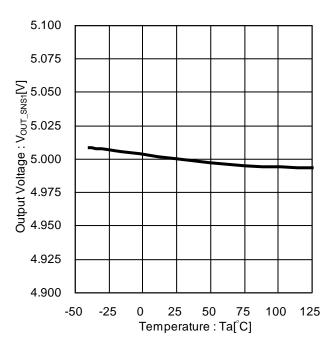
Figure 12. Output Voltage vs Temperature (BD9P155MUF-C)
