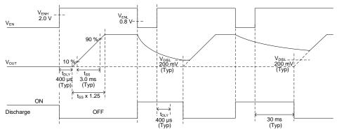
Figure 33. Enable ON/OFF Timing Chart
