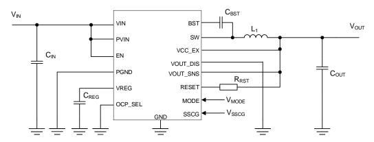
Figure 2. Application Circuit without Discharge Function (BD9P135MUF-C, BD9P155MUF-C)
