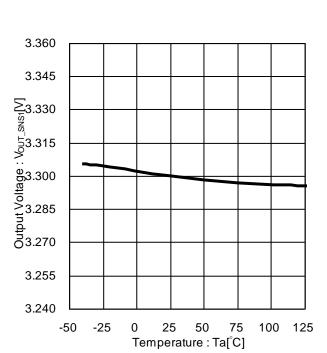
Figure 11. Output Voltage vs Temperature (BD9P135MUF-C)
