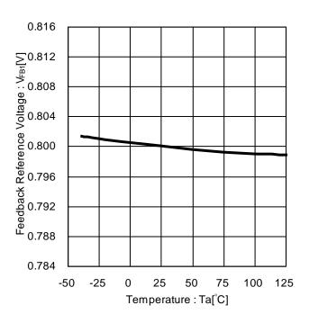
Figure 10. Feedback Reference Voltage vs Temperature (BD9P105MUF-C)
