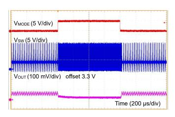
Figure 66. MODE ON/OFF Response (V<sub>IN</sub> = 12 V, I<sub>OUT</sub> = 50 mA)
