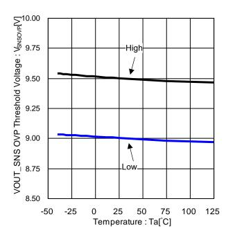
Figure 27. VOUT\_SNS OVP Threshold Voltage vs Temperature (BD9P105MUF-C)
