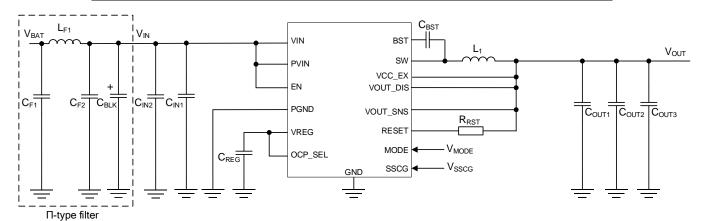
Figure 62. Reference Circuit 2
