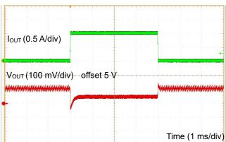
Figure 80. Load Response 1 (V<sub>IN</sub> = 12 V, V<sub>MODE</sub> = 5 V, I<sub>OUT</sub> = 0 A to 1 A)
