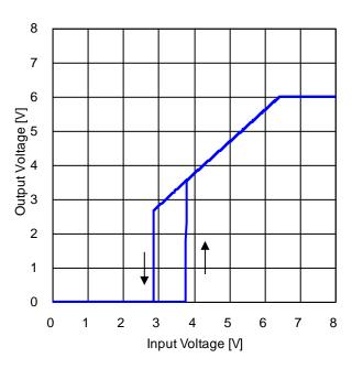
Figure 59. Output Voltage vs Input Voltage 2  $(R_{LOAD} = 6 \Omega)$
