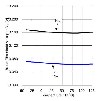
Figure 24. Reset Threshold Voltage vs Temperature (BD9P135MUF-C)
