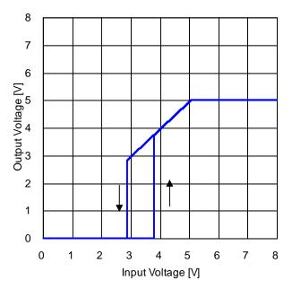
Figure 84. Output Voltage vs Input Voltage 1  $(R_{LOAD} = 500 \Omega)$
