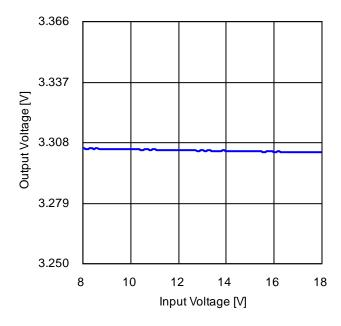
Figure 73. Line Regulation (I<sub>OUT</sub> = 1 A)
