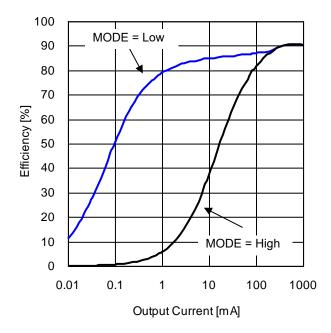
Figure 50. Efficiency vs Output Current  $(V_{IN} = 12 V)$
