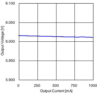
Figure 61. Load Regulation (V<sub>IN</sub> = 12 V)
