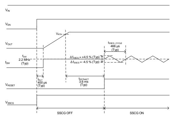
Figure 37. Spread Spectrum Function
