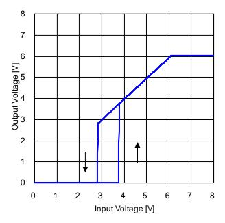
Figure 58. Output Voltage vs Input Voltage 1  $(R_{LOAD} = 600 \Omega)$
