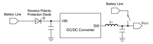
Figure 46. VOUT Shorted to Battery Line
