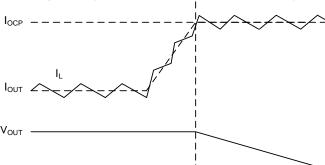
Figure 40. Over Current Protection
