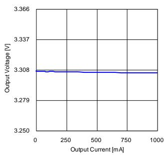
Figure 74. Load Regulation (V<sub>IN</sub> = 12 V)
