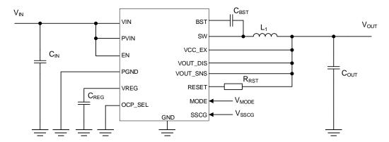
Figure 1. Application Circuit with Discharge Function (BD9P135MUF-C, BD9P155MUF-C)
