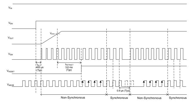
Figure 35. External Synchronization Function
