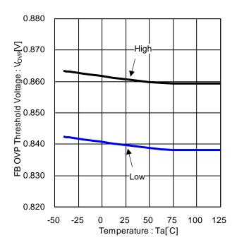
Figure 26. FB OVP Threshold Voltage vs Temperature (BD9P105MUF-C)
