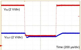
Figure 82. Line Response 1 (V<sub>IN</sub> = 16 V to 8 V, I<sub>OUT</sub> = 1 A)
