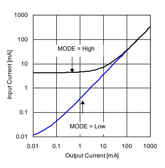
Figure 64. Input Current vs Output Current (V<sub>IN</sub> = 12 V)
