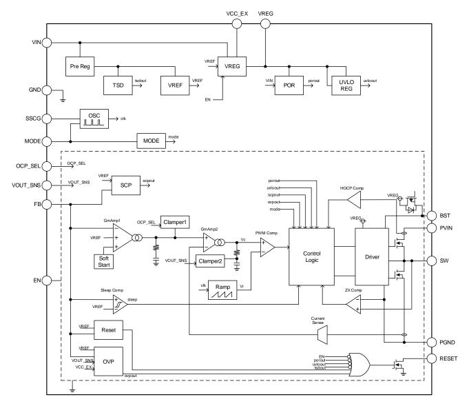
Figure 7. Block Diagram (BD9P105MUF-C)
