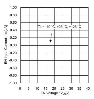
Figure 16. EN Input Current vs EN Voltage
