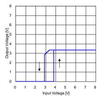
Figure 71. Output Voltage vs Input Voltage 1  $(R_{LOAD} = 330 \Omega)$
