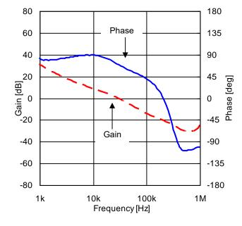
Figure 78. Frequency Characteristic (V<sub>IN</sub> = 12 V, I<sub>OUT</sub> = 0.5 A)
