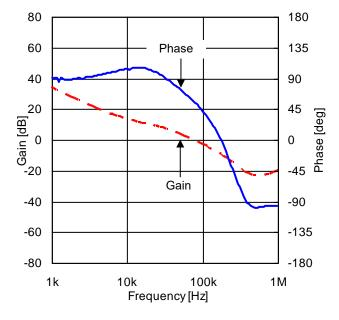
Figure 65. Frequency Characteristic (V<sub>IN</sub> = 12 V, I<sub>OUT</sub> = 0.5 A)
