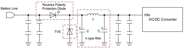
Figure 88. Automotive Power Supply Line Circuit
