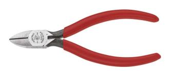
Tapered nose for easy working in confined areas and close tip cutting. Short jaws and beveled cutting edges permit close cutting of wire. Induction-hardened cutting knives for long life. Hot-riveted joint ensures smoot action and not handle wobble. Plastic-dipped handles for comfort and ease of identification. Custom, US-made tool steel.
