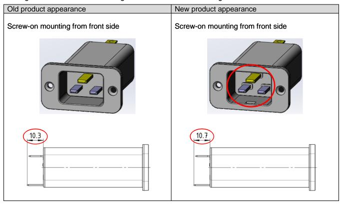
As the V-Lock notch and material for enhanced glow wire tests will be standard features, the material numbers with index .21 are obsolete and will be replaced by the standard numbers:
