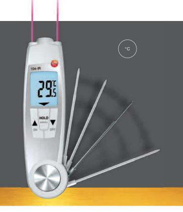
The testo 104-IR is a waterproof (IP65) penetration thermometer combined with an infrared sensor for noncontact temperature measurement. It can be used for all sorts of applications in the food sector. The testo 104-IR scans the surface temperature of individual foods or entire goods pallets without contact, particularly in the Incoming Goods department. If a limit value is exceeded or undershot, the hinged penetration probe is also able to measure the core temperature.
