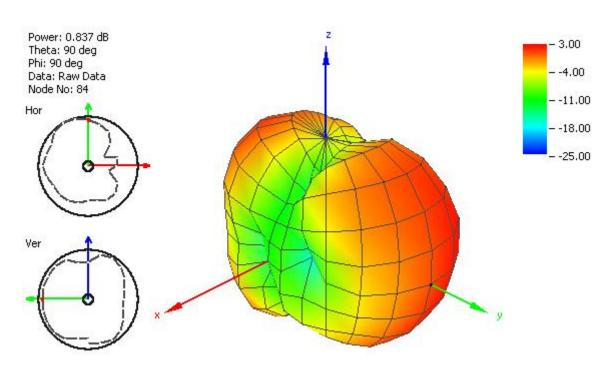
Figure 17. Radiation Pattern at 2600 MHz of FXUB66 UWB Antenna.
