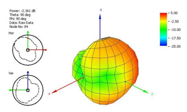
Figure 11. Radiation Pattern at 1575 MHz of FXUB66 UWB Antenna.
