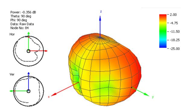
Figure 14. Radiation Pattern at 1950 MHz of FXUB66 UWB Antenna.
