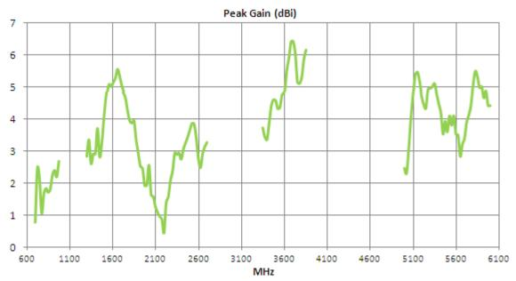
Figure 5. Peak Gain of FXUB66 UWB Antenna.
