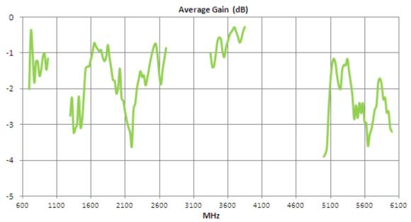
Figure 6. Average Gain of FXUB66 UWB Antenna.
