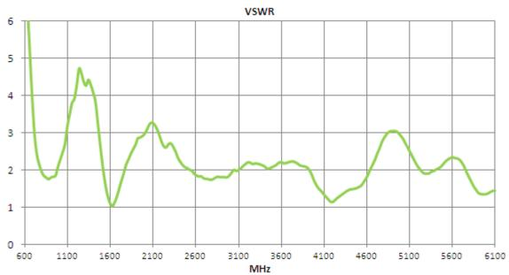
Figure 3. VSWR of FXUB66 UWB Antenna.
