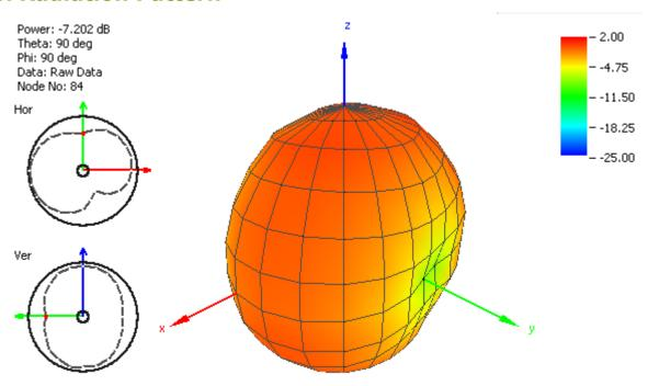
Figure 7. Radiation Pattern at 750 MHz of FXUB66 UWB Antenna.
