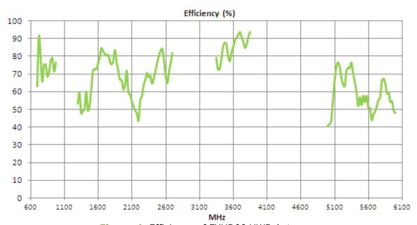
Figure 4. Efficiency of FXUB66 UWB Antenna.
