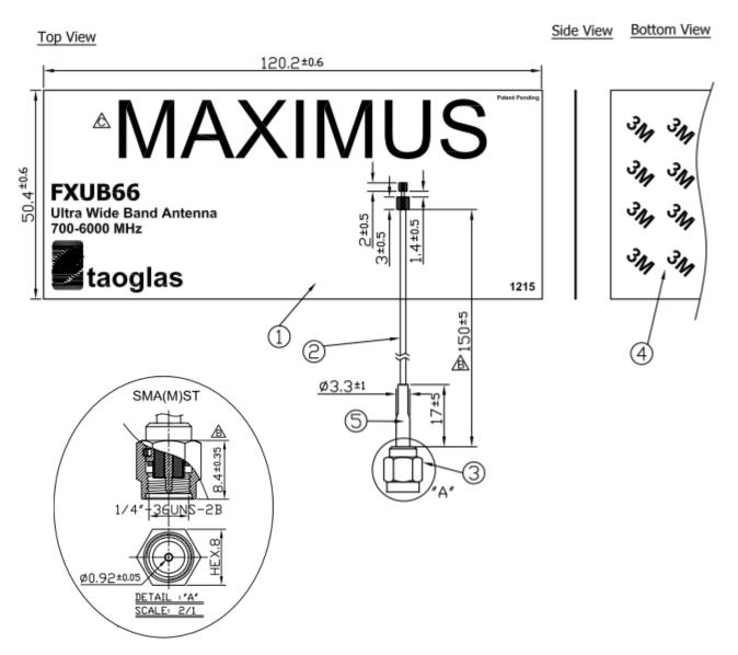
Figure 20. Mechanical drawing of FXUB66 UWB Antenna.
