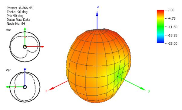
Figure 8. Radiation Pattern at 850 MHz of FXUB66 UWB Antenna.
