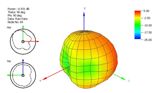
Figure 12. Radiation Pattern at 1750 MHz of FXUB66 UWB Antenna.
