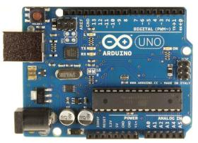
The Uno differs from all preceding boards in that it does not use the FTDI USB-to-serial driver chip. Instead, it features the Atmega16U2 (Atmega8U2 up to version R2) programmed as a USB-to-serial converter.
