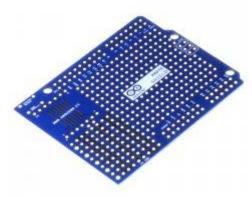
It has 12 standard TinkeKit 3pin connectors. The 6 labeled **IO** through **I5** are **Analog Inputs**. The ones labeled **OO** through **O5** are **Analog Outputs** connected to the PWM capable outputs of the Arduino Board (it is possible to change these to Digital Inputs, in which case they will report either HIGH or LOW, but nothing in between).
