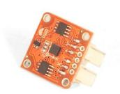
An **accelerometer** is a device that measures acceleration. It is very common in consumer electronics such as portable electronic devices and video game controllers to detect movement using accelerometers.
