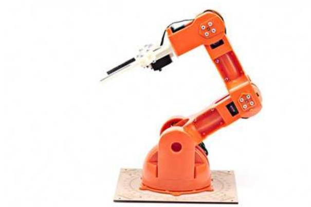
You can assemble your BRACCIO in a multitude of ways. Because it is designed for versatility, the BRACCIO can also support various objects on the end of the arm. The included BRACCIO shield allows you to hook up the servos directly to your Arduino board.
