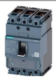
CIRCUIT BREAKER 3VA1 IEC FRAME 160 BREAKING CAPACITY CLASS H ICU=70KA @ 415 V 3-POLE, LINE PROTECTION TM220, ATFM, IN=160A OVERLOAD PROTECTION IR=112A ...160A SHORT CIRCUIT PROTECTION II=10 X IN BUSBAR CONNECTION
