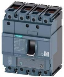
CIRCUIT BREAKER 3VA1 IEC FRAME 160 BREAKING CAPACITY CLASS S ICU=36KA @ 415 V 4-POLE, LINE PROTECTION TM240, ATAM, IN=25A OVERLOAD PROTECTION IR=17,5A ...25A SHORT CIRCUIT PROTECTION II=5...10 X IN NEUTRAL PROTECTION 100% CABLE CONNECTION
