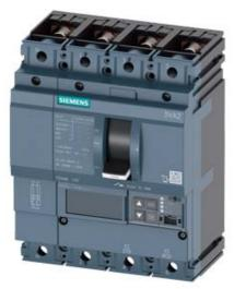
CIRCUIT BREAKER 3VA2 IEC FRAME 100 BREAKING CAPACITY CLASS H ICU=85KA @ 415 V 4POLE, LINE PROTECTION ETU550, LSI, IN=63A OVERLOAD PROTECTION IR=25A ...63A SHORT CIRCUIT PROTECTION ISD=0,6..10X IN, II=1,5..12X IN NEUTRAL PROTECTION ADJUSTABLE (OFF, UPTO 160%) BUSBAR CONNECTION
