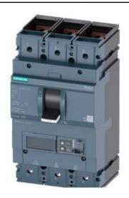
CIRCUIT BREAKER 3VA2 IEC FRAME 400 BREAKING CAPACITY CLASS M ICU=55KA @ 415 V 3-POLE, LINE PROTECTION ETU560, LSIG, IN=400A OVERLOAD PROTECTION IR=160A ...400A SHORT CIRCUIT PROTECTION ISD=0,6..10X IN, II=1,5..10X IN NEUTRAL PROTECTION OPTIONAL WITH EXT. CT;UPTO 160% GROUND-FAULT, SWITCHABLE IG=0,2... 1 X IN, TG=0,05-0,8MS BUSBAR CONNECTION
