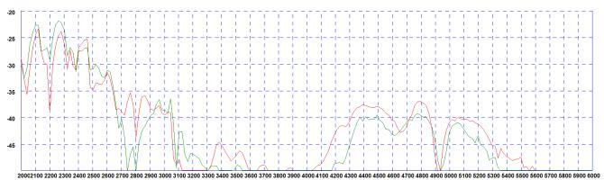
\*Isolation measured with no whip and 5m (16') of CS29 cable Red Plot = 600x600mm (2' X2') ground plane Green Plot = no ground plane
