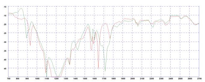
\*Isolation measured with no whip and 5m (16') of CS29 cable Green Plot = 600x600mm (2' X2') ground plane Red Plot = no ground plane Typical Isolation - WiFi Elements 4&5\*
