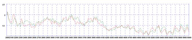
\*VSWR measured with no whip and 5m (16') of CS32 cable
