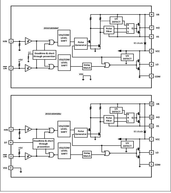
Figure 2 Block diagrams
