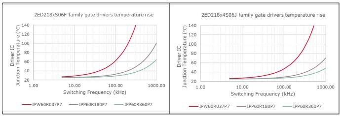
\*Assumptions for above curves:  $T_a = 25 \text{ °C}$ ,  $V_{BUS} = 400 \text{ V}$ ,  $V_{CC} = 12 \text{ V}$ ,  $R_{gon} = 10 \Omega$ ,  $R_{goff} = 5\Omega$
