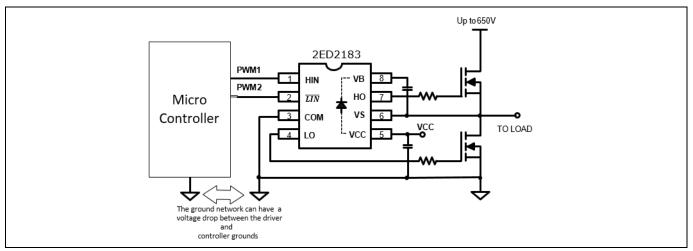
Figure 15 Negative voltage tolerance on inputs of upto –5 V
