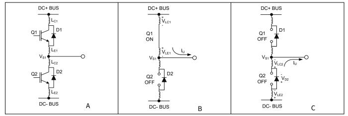
Figure 18 Figure A shows the Parasitic Elements. Figure B shows the generation of V<sub>s</sub> positive. Figure C shows the generation of V<sub>s</sub> negative
