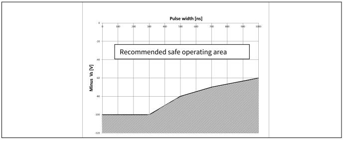
Figure 19 Negative VS transient SOA for 2ED2183(4)S06F(J) @ VBS=15 V
