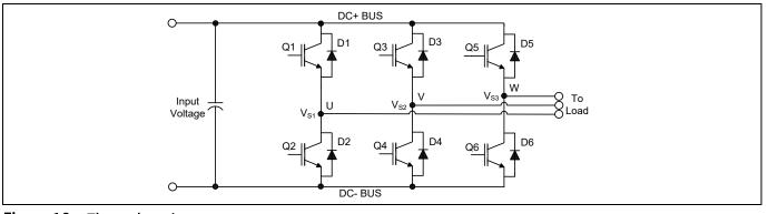
Figure 16 Three phase inverter
