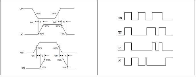
Figure 6 Switching timing diagram
