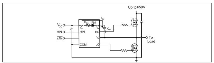
Figure 14 Half bridge bootstrap circuit in 2ED218x
