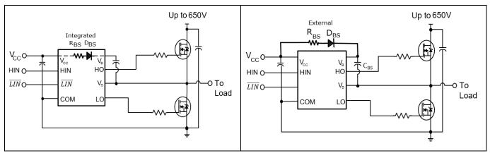
Figure 12 2ED218x with integrated components Figure 13 Standard bootstrap gate driver
