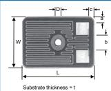
Fixing hole is located centrally except on WDBR1/2 where the dimension from the edge by the terminations to the mounting hole centre is 16.68mm.
