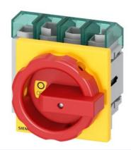
SENTRON, Molded case switch 3LD5 UL, Emergency switching-off, 4-pole, certified according to UL489 UL60947-4-1 and IEC60947-3, UL: 60A, SCCR 50kA at 480VAC, Operating power at 480VAC 3-phase: 40hp, IEC: 63A, Operating power at AC-23A at 400V: 30kW, front-mounted, rotary operating mechanism, red/yellow, 4-hole mounting of the handle, incl. terminal covers for the infeed side
