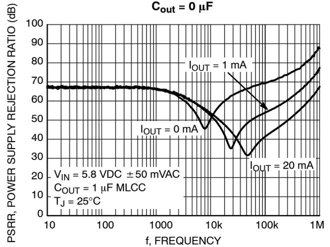
Figure 13. Power Supply Rejection Ratio
