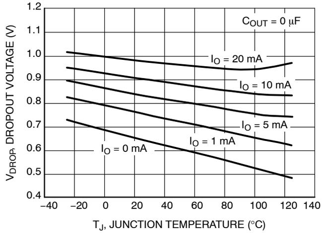
Figure 5. Dropout Voltage
