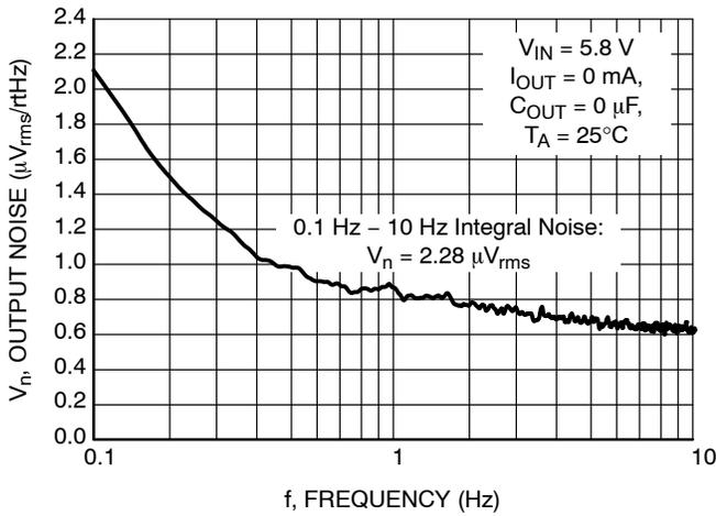
Figure 16. Output Voltage Noise 0.1 Hz - 10 Hz
