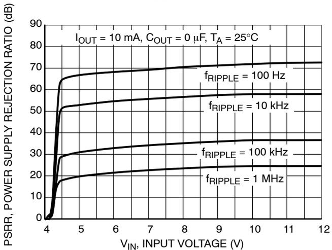
Figure 14. Power Supply Rejection Ratio vs. Input Voltage
