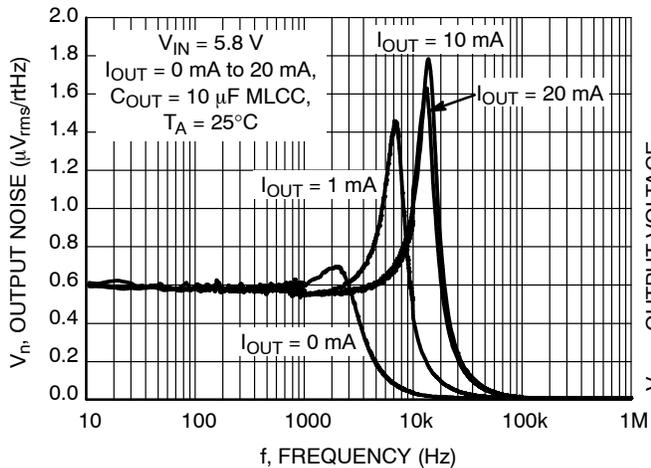
Figure 20. Output Voltage Noise 10 Hz - 1 MHz
