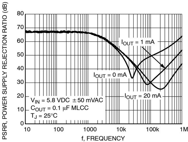
Figure 12. Power Supply Rejection Ratio
