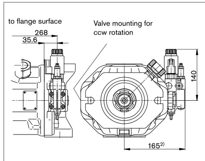
1) ER7.: 379 mm when using a sandwich plate pressure reducing valve.
