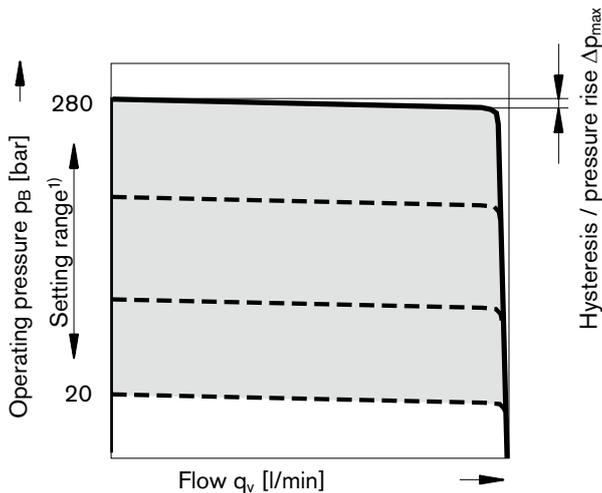
1) In order to prevent damage to the pump and the system, this setting range is the permissible setting range and must not be exceeded. The range of possible settings at the valve are greater.
