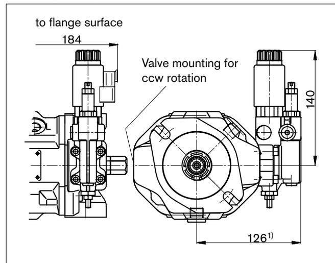
1) ER7.: 161 mm if using a sandwich plate pressure reducing valve.
