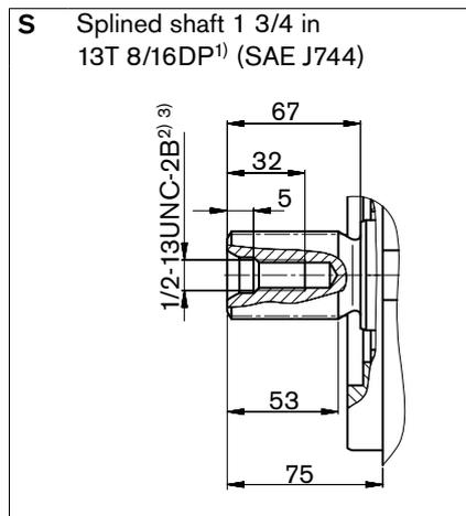
1) ANSI B92.1a, 30° pressure angle, flat root, side fit, tolerance class 5
