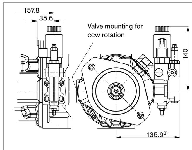
1) ER7.: 260 mm when using a sandwich plate pressure reducing valve.
