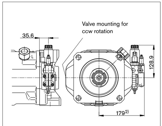
1) ER7.: 384 mm when using a sandwich plate pressure reducing valve.
