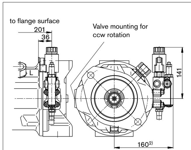
1) ER7.: 314 mm when using a sandwich plate pressure reducing valve.
