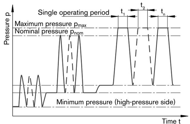
Total operating period =  $t_1 + t_2 + \dots + t_n$
