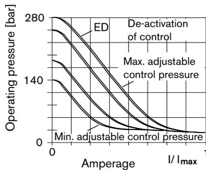
Hysteresis of the static current-pressure characteristic < 3 bar
