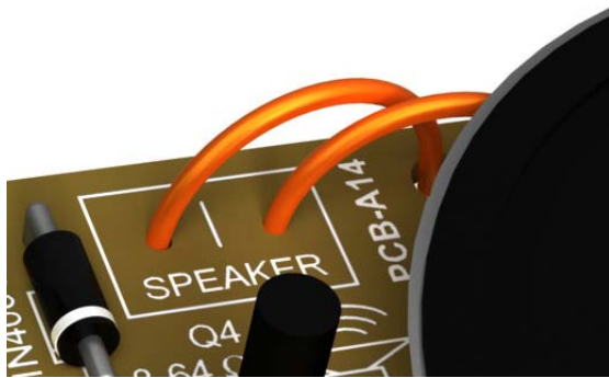
◀ Loudspeaker wired to the board.
