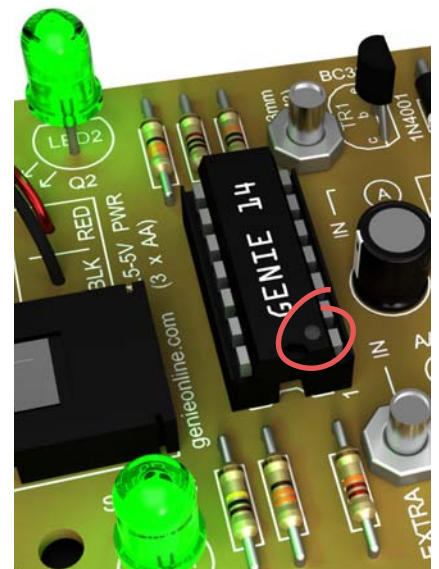
▶ The GENIE chip inserted into the 14-pin chip socket. The pin 1 'dot' is highlighted.
