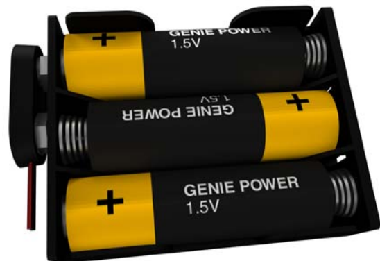
Battery box showing all three cells inserted and the battery clip connected.
