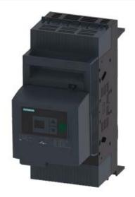
FUSE-SWITCH-DISCONNECTOR 3-POLE, NH000, 160A 60MM BUSBAR SYSTEM COVER LEVEL 32/70 MM BOX TERMINAL FUSE MONITORING ELECTRONIC, EFM 20
