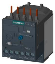
OVERLOAD RELAY 0.32...1.25 A FOR MOTOR PROTECTION SIZE S00, CLASS 20 CONTACTOR ASS. MAIN CIRCUIT: SCREW CONN. AUX.CIRCUIT: SCREW CONN. MANUAL-AUTOM.-RESET
