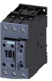
CONTACTOR, AC3:18.5KW/400V, 1NO+1NC, 24V AC 50/60HZ, 3-POLE, SIZE S2, SCREW TERMINAL
