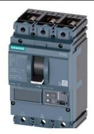
CIRCUIT BREAKER 3VA2 IEC FRAME 100 BREAKING CAPACITY CLASS L ICU=150KA @ 415 V 3POLE, LINE PROTECTION ETU860, LSIG, IN=100A OVERLOAD PROTECTION IR=40A ...100A SHORT CIRCUIT PROTECTION ISD=0,6..10X IN, II=1,5..12X IN NEUTRAL PROTECTION OPTIONAL WITH EXT. CT,UPTO 160% GROUNDFAULT, SWITCHABLE IG=0,2... 1 X IN, TG=0,050,8MS BUSBAR CONNECTION
