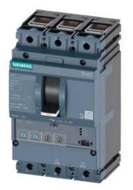
CIRCUIT BREAKER 3VA2 IEC FRAME 160 BREAKING CAPACITY CLASS H ICU=85KA @ 415 V 3POLE, LINE PROTECTION ETU330, LIG, IN=100A OVERLOAD PROTECTION IR=40A ...100A SHORT CIRCUIT PROTECTION II=1,5...12 X IN GROUNDFAULTPROTECTION IG=0,2... 1 X IN, TG=0,1/0,3MS CABLE CONNECTION
