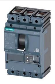
CIRCUIT BREAKER 3VA2 IEC FRAME 160 BREAKING CAPACITY CLASS H ICU=85KA @ 415 V 3POLE, LINE PROTECTION ETU560, LSIG, IN=160A OVERLOAD PROTECTION IR=64A ...160A SHORT CIRCUIT PROTECTION ISD=0,6..10X IN, II=1,5...10X IN NEUTRAL PROTECTION OPTIONAL WITH EXT. CT,UPTO 160% GROUNDFAULT, SWITCHABLE IG=0,2... 1 X IN, TG=0,050,8MS CABLE CONNECTION
