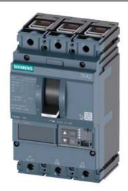
CIRCUIT BREAKER 3VA2 IEC FRAME 160 BREAKING CAPACITY CLASS L ICU=150KA @ 415 V 3POLE, LINE PROTECTION ETU860, LSIG, IN=25A OVERLOAD PROTECTION IR=10A ...25A SHORT CIRCUIT PROTECTION ISD=0,6..10X IN, II=1,5..12X IN NEUTRAL PROTECTION OPTIONAL WITH EXT. CT,UPTO 160% GROUNDFAULT, SWITCHABLE IG=0,2... 1 X IN, TG=0,050,8MS CABLE CONNECTION
