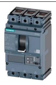
CIRCUIT BREAKER 3VA2 IEC FRAME 160 BREAKING CAPACITY CLASS M ICU=55KA @ 415 V 3POLE, LINE PROTECTION ETU560, LSIG, IN=40A OVERLOAD PROTECTION IR=16A ...40A SHORT CIRCUIT PROTECTION ISD=0,6..10X IN, II=1,5...12X IN NEUTRAL PROTECTION OPTIONAL WITH EXT. CT,UPTO 160% GROUNDFAULT, SWITCHABLE IG=0,2... 1 X IN, TG=0,050,8MS CABLE CONNECTION
