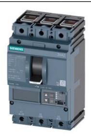
CIRCUIT BREAKER 3VA2 IEC FRAME 160 BREAKING CAPACITY CLASS H ICU=85KA @ 415 V 3POLE, LINE PROTECTION ETU560, LSIG, IN=40A OVERLOAD PROTECTION IR=16A ...40A SHORT CIRCUIT PROTECTION ISD=0,6..10X IN, II=1,5...12X IN NEUTRAL PROTECTION OPTIONAL WITH EXT. CT,UPTO 160% GROUNDFAULT, SWITCHABLE IG=0,2... 1 X IN, TG=0,050,8MS CABLE CONNECTION
