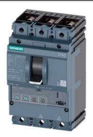
CIRCUIT BREAKER 3VA2 IEC FRAME 160 BREAKING CAPACITY CLASS C ICU=110KA @ 415 V 3POLE, LINE PROTECTION ETU330, LIG, IN=40A OVERLOAD PROTECTION IR=16A ...40A SHORT CIRCUIT PROTECTION II=1,5...12 X IN GROUNDFAULTPROTECTION IG=0,2... 1 X IN, TG=0,1/0,3MS BUSBAR CONNECTION
