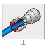
. To make sure that the fitting is properly connected to the tube, pull it once. After pulling, insert a spanner under the collet and push the tube into the fitting once more for a complete insertion.
