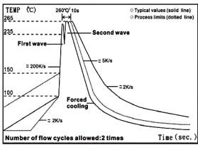
IR Reflow Soldering
