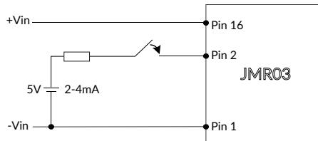
Module "On" if pin 2 is open circuit
