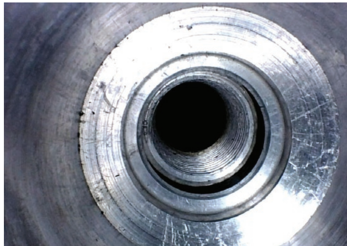
Photo above: Spark plug port inspection
