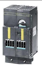
F-RS1E-X FOR ET 200S FAILSAFE REVERSING STARTER SETTING RANGE 2.4...16A, MECHANICAL SWITCHING, ELECTRONIC PROTECTION, AC-3, TO 7.5KW/400V, CAN BE EXPANDED, FOR BRAKE CONTROL MODULE FOR 2DI CONTROL MODULE
