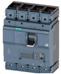
CIRCUIT BREAKER 3VA2 IEC FRAME 400 BREAKING CAPACITY CLASS M ICU=55KA @ 415 V 4-POLE, LINE PROTECTION ETU850, LSI, IN=250A OVERLOAD PROTECTION IR=100A ...250A SHORT CIRCUIT PROTECTION ISD=0,6..10X IN, II=1,5..12X IN NEUTRAL PROTECTION ADJUSTABLE (OFF, UPTO 160%) BUSBAR CONNECTION
