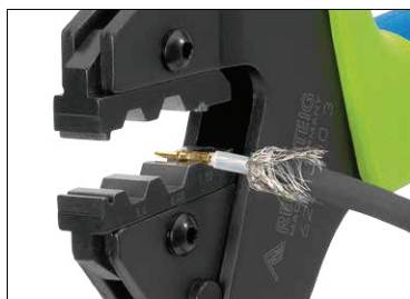
Innenleiter-Crimp Inner conductor crimp
