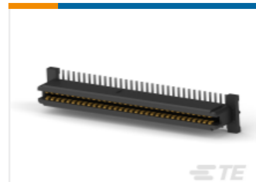
TE Part #5146893-2 Free Height Receptacle Conn: Board-Board, Vertical, 84, 1mm
