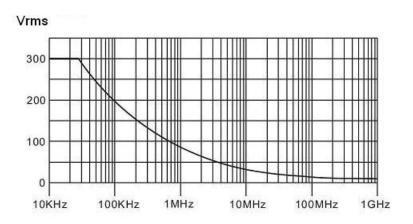
Figure 5. N2862B/63B/89A/90A voltage derating curve
