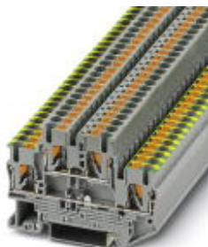
Protective conductor double-level terminal block, Connection type: Push-in connection, Cross section: 0.14 mm 2 - 4 mm 2 , AWG: 26 - 12, Width: 5.2 mm, Color: gray, Mounting type: NS 35/7,5, NS 35/15
