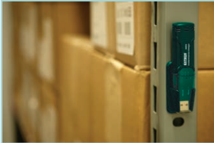
Monitors Temperature level in a warehouse or storage room.
