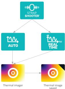
In STRAP**SHOOTER® REAL TIME** or **AUTO** mode, select THERMAL icon and wait some seconds to have a stable thermal image (wait after first shutter activation):
