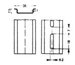
Fixing holes Dimension b to specs. (dia. 3.5/4.5/5.5/7) Dimension  $I_2$  to specs. Dimension  $I_1$  to 2 m
