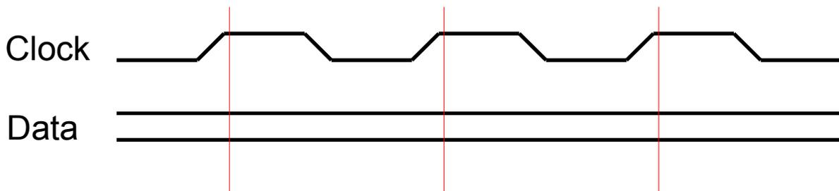
Fig. 4: Sampling with synchronous clock
