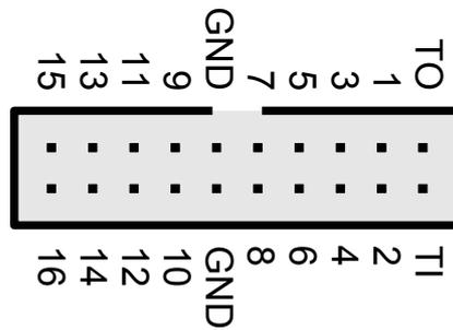
Fig. 1: Target connector
