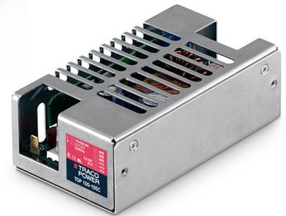
The new TOP-100 Series AC/DC Power Supplies feature the highest power rating in the industry standard 2.0" x 4.0" (50.8 x 101.6 mm) footprint. They can supply up to 100 W output power with convection cooling over an industrial operating temperature range of -25°C to +50°C. This performance could be realized by a state of the art design providing an extremely high efficiency of >90 % which eliminates the need for a dedicated power supply cooling fan.
