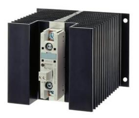
SEMI-COND. CONTACTOR 3RF2,1-PH. AC 51 70A/AC15 27.5A 40 DEG. C 48-600 V / 110-230 V AC INSTANTANEOUS SWITCHING
